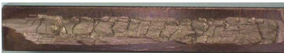
Figure 2 – Galled AISI 1020 carbon steel samples after a single sliding stroke under a contact stress of 70 Mpa. Width of sample is 1.27 cm.
